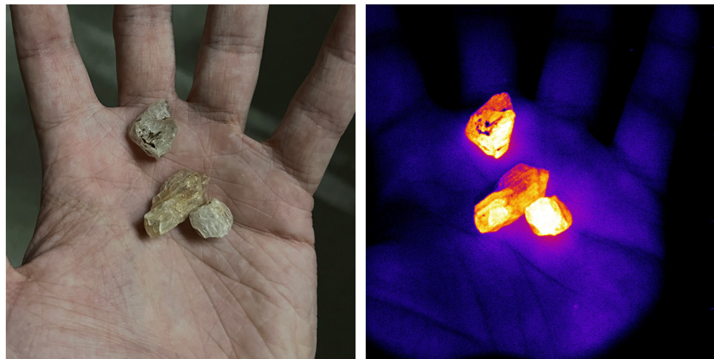
LHS: three sodium-rich feldspar pebbles under white light RHS: imaged in their NIR fluorescence
