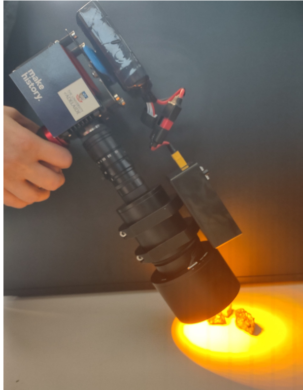
Fluorine mineral sensor in both 1U cubesat and handheld formats
